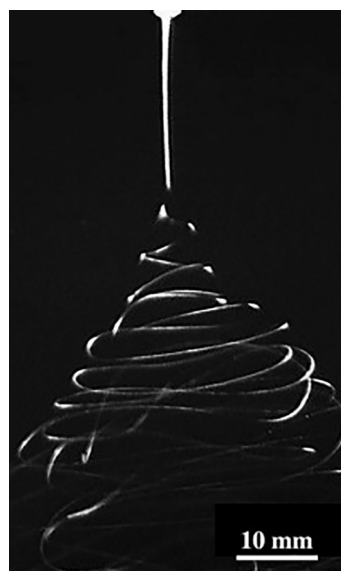
Figure 1.3. Digital photo of an electrospinning solution jet, including a stable jet and jet whipping stage. Reproduced with permission from Elsevier [39].
