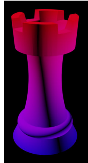
Figure A.3: A "meta" material is defined in the material palette as a functional combination of two previously defined materials. This enables smooth gradients and arbitrary 3D material distributions within an object.
